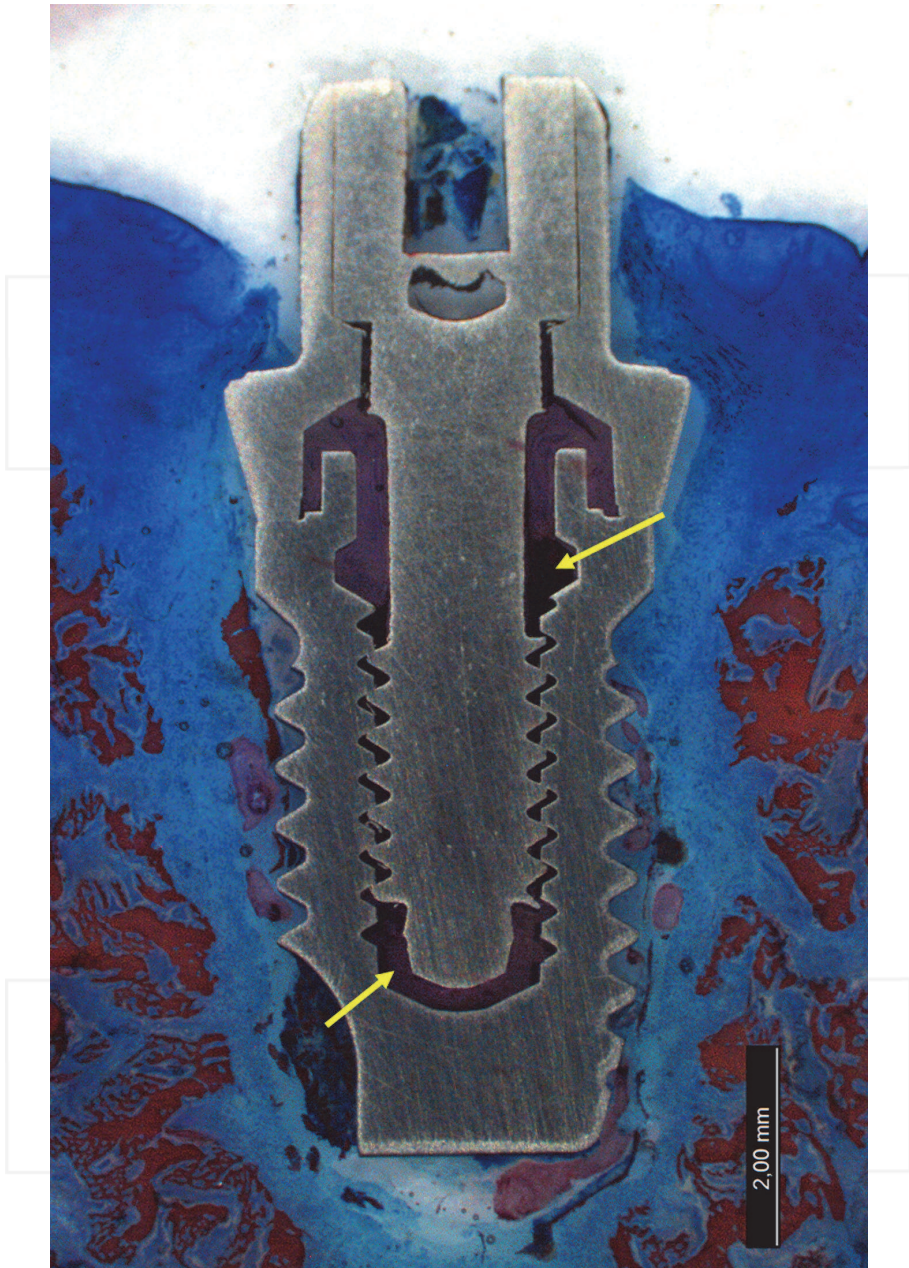
Fig. 1. Histological Photomicrograph showing the gaps and hollow spaces (arrows) resulted from the poor adaptation of the implant and prosthetic components in the two-part implant systems (MKIII TiUnit and it respective abutment, Nobel Biocare- regular external hexagonal platform with 3.75 mm in diameter and 7 mm in length).
