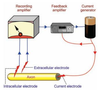
FIGURE 136.2: Voltage clamping
