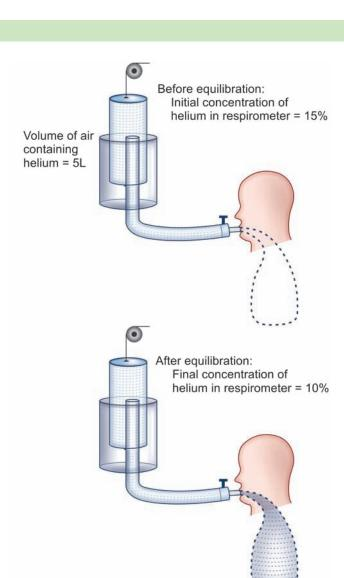
FIGURE 121.4: Measurement of functional residual capacity by using helium
