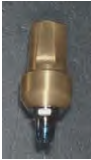
Figure 5.12. Pre-machined titanium abutment as received from the manufacturer. This GingiHue ® Post (IAPP454G) was made for a 4.1 mm diameter, internal connection implant. It has a 5 mm emergence profile and a 4 mm collar height.
