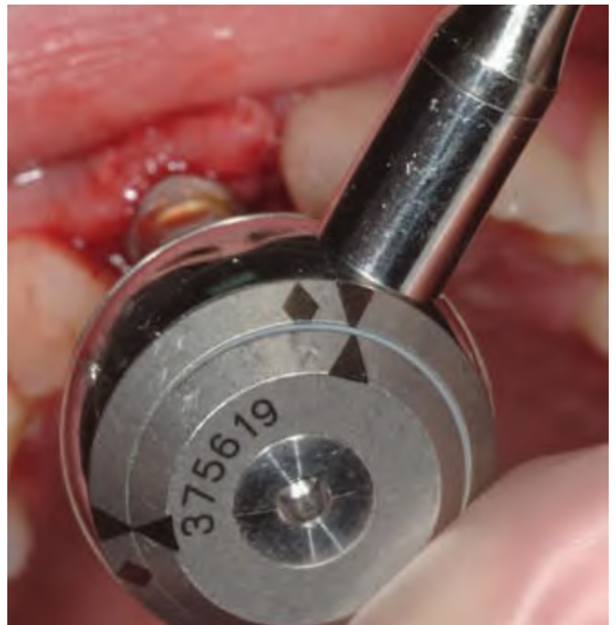
Figure 9.20. Occlusal view of the Restorative Torque Indicator (RTI2035) that demonstrated 20 Ncm of torque (triangle to triangle).
