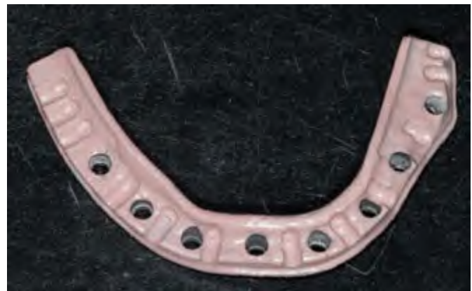
Figure 7.44. The CAD/CAM mandibular framework was milled and silicoated prior to the clinical try-in appointment.
