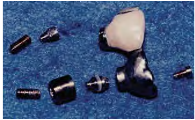
Figure 5.4. Laboratory view of broken implant restorative components. This prosthesis was inserted in 1989. There was micro movement among the implant restorative components that was below the consciousness of the patient. The movement continued until such time that the abutment screws fractured.
