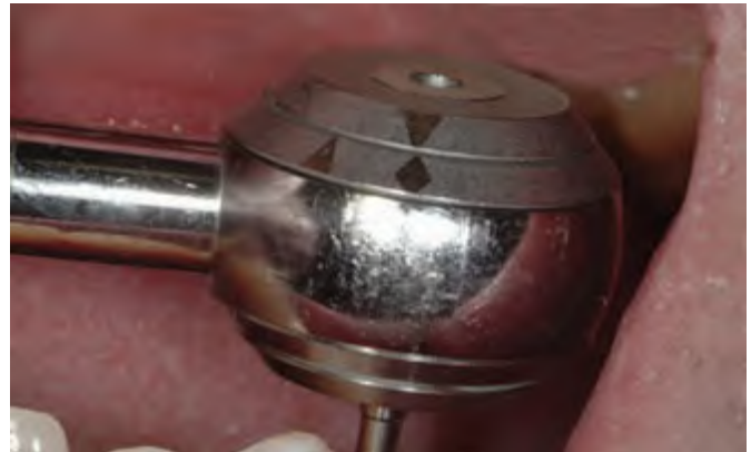
Figure 7.59. The head of a Restorative Torque Indicator. The triangle to diamond indicated that 35 Ncm of preload was generated to the abutment screw.
