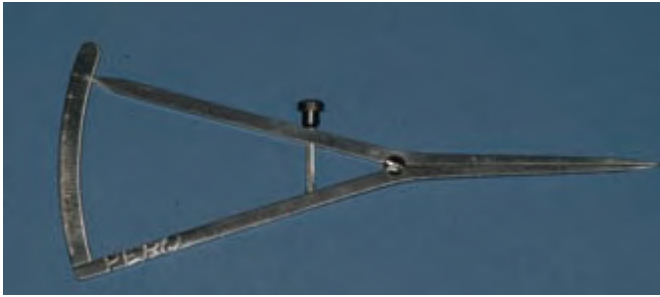
Figure 8.5. Castroviejo caliper used to measure the amount of inter-occlusal distance available for osteotomy and implant placement.
