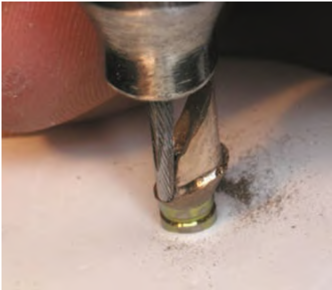
Figure 2.78. A custom UCLA Abutment was developed in wax and cast in a noble alloy. It was milled on a surveyor for minimal axial wall taper. The sub-gingival portions were waxed to fit into the peri-implant space around the implant analog.
