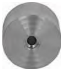
Figure 6.32. External hex blank of titanium alloy prior to milling the CAD/CAM abutments.
