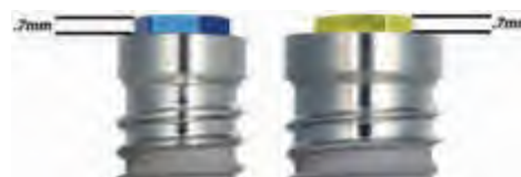
Figure 2.3. Profile view of OSSEOTITE ® external hex implant. Vertical measurement of external hex measures 0.7 mm. (4.1 mm restorative platform left; 5.0 mm restorative platform right).
