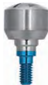
Figure 5.18. Profile view of a healing abutment for a 4.1 mm implant restorative platform, 6 mm emergence profile, and 4 mm collar height for the OSSEOTITE ® Certain ® implant system (ITHA464).
