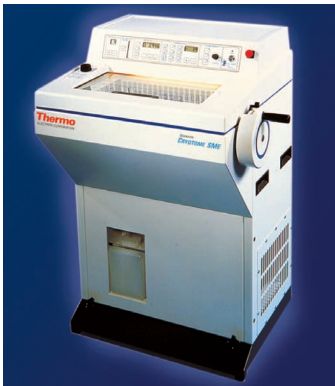
Figure 2.4 ♦ Cryostat for cutting sections by freezing technique (Cryotones). (Thermo Shandon, UK). Courtesy: Towa Optics (India) Pvt. Ltd., New Delhi.
