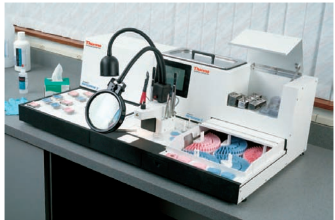
Figure 2.2 ◆ Tissue embedding centre for paraffin technique (HistoCentre). (Thermo Shandon, UK). Courtesy: Towa Optics (India) Pvt. Ltd., New Delhi.
