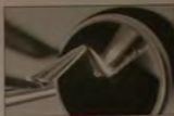
Fig 6-50a Front-surface mirror. Any object touching the mirror, such as the tips of the cotton forceps, will appear to be touching itself.
