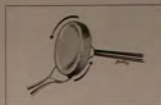
Fig 6-49 Sharpening a discoid spoon with a rotating sharpening stone. A discoid spoon may also be sharpened on a flat stone; the blade is rotated as it is pulled with the cutting edge forward. If the face is ground with a rotating stone, the blade will be thinned and could be more likely to break during use.
