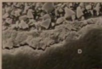
Fig 8-104b Dicor glass ceramic (D) was etched for 60 seconds with 10% ammonium bifluoride and luted with Dicor MGC (C) without ultrasonic cleaning.
