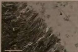
Fig 8-93 Transmission electron photomicrograph of the interface between a two-step self-etch adhesive (Clearfil SE, Kuraray) and enamel. Note the superficial interaction of the adhesive (A) with the enamel (E). Bar = 500 nm.
