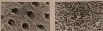
Figs 8-51a and 8-51b Field-emission scanning electron photomicrographs showing the effect of 36% phosphoric acid (DeTrey Etch) on dentin (top view). Note the deposition of silica particles that remained from the acid etchant [thickener] despite it having been thoroughly rinsed off. Nevertheless, higher magnification (b) disclosed that the interfibrillar spaces remained penetrable for resin. Bar = 2 \mu\text{m} (a) and 0.5 \mu\text{m} (b).
