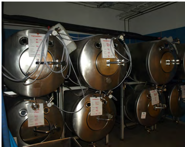
Figure 4.18 Fermentation of grape juice to make wine produces \text{CO}_2 as a byproduct. Fermentation tanks have valves so that pressure inside the tanks can be released.
