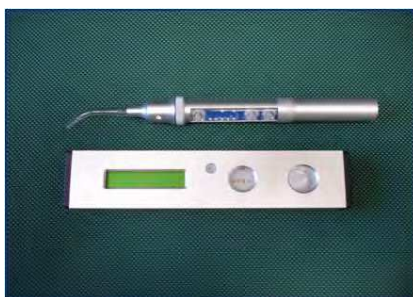
Fig. 8. Fiber-optic transillumination device (DioPower Lamp)
