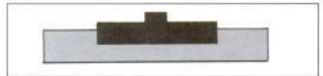
Fig. 8.13: Fusing the male mounting plate on a plexiglass
