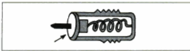
Fig. 22.83: Collar of the casing that controls the movement of the nipple out of the casing
