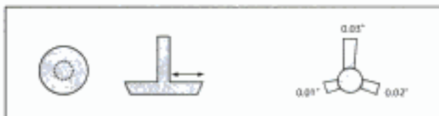
Fig. 18.7c: Ney undercut gauge (available in different sizes). Jelenko undercut gauge (single gauge can be used to locate undercuts of different sizes)
