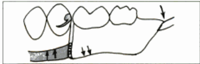
Fig. 18.261: Stress breakers can be added to the junction between the tooth supported portion and tissue supported portion of the denture to avoid leverage forces
