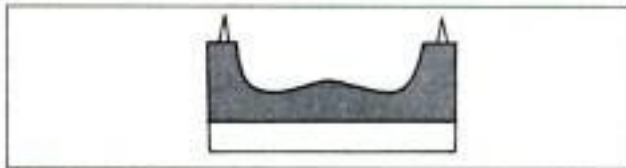
Fig. 8.23a: Box plaster showing conical projections with respect to the land area of the cast
