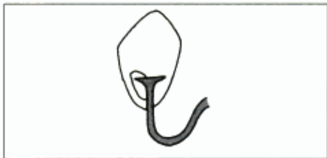
Fig. 18.180: Retentive finger that engages an undercut
