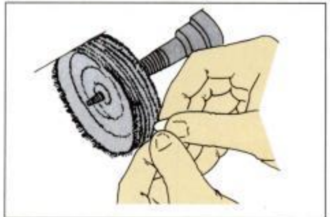
Fig. 32.12: Axial surfaces are polished using white polishing compound on a muslin rag wheel
