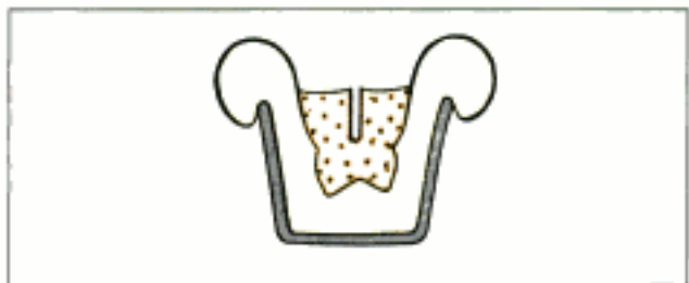
Fig. 33.5: In the post pour technique, holes are drilled into the set first pour to position the pins
