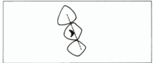
Fig. 19.21: The cingulum rest seat should be gingival to the point of contact (dotted line)
