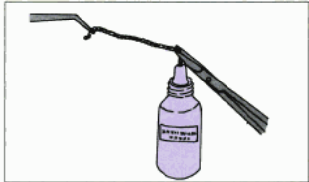
Fig. 31.6: Retracting the cord from dispensing bottle
