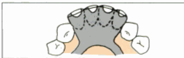
Fig. 18.142b: When multiple incisal rests are placed, each. One is not individually connected to the major connector. Instead they are interconnected with a metal plate which is connected to the major connector
