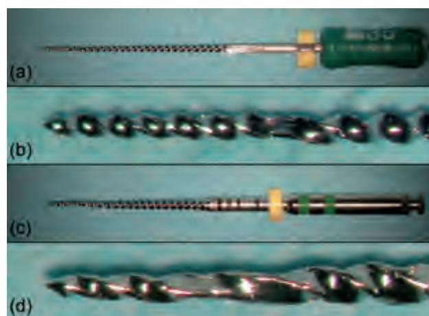
Fig. 11.23 (a, c) Hand and rotary files showing unwinding of the flutes. (b, d) A detailed view on the area with deformation.
