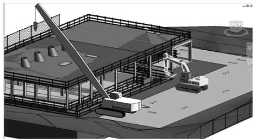
Figure 1. 3D model of structure and safety elements—Revit.
