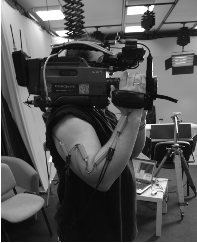
Figure 1. An example of an upper-limb measurement using goniometers and torsionmeters attached to worker skin (Source: Turkiewicz 2013).
