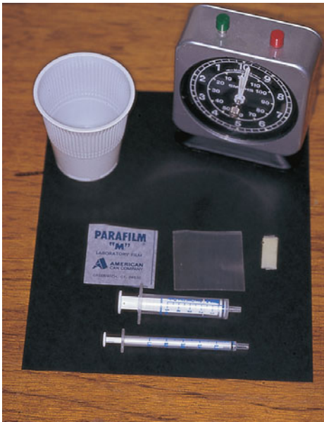
Figure 3.23. Paraffin film, paper cup, timer and disposable graduated syringes (1 and 5 ml) for measurement of salivary flow.
