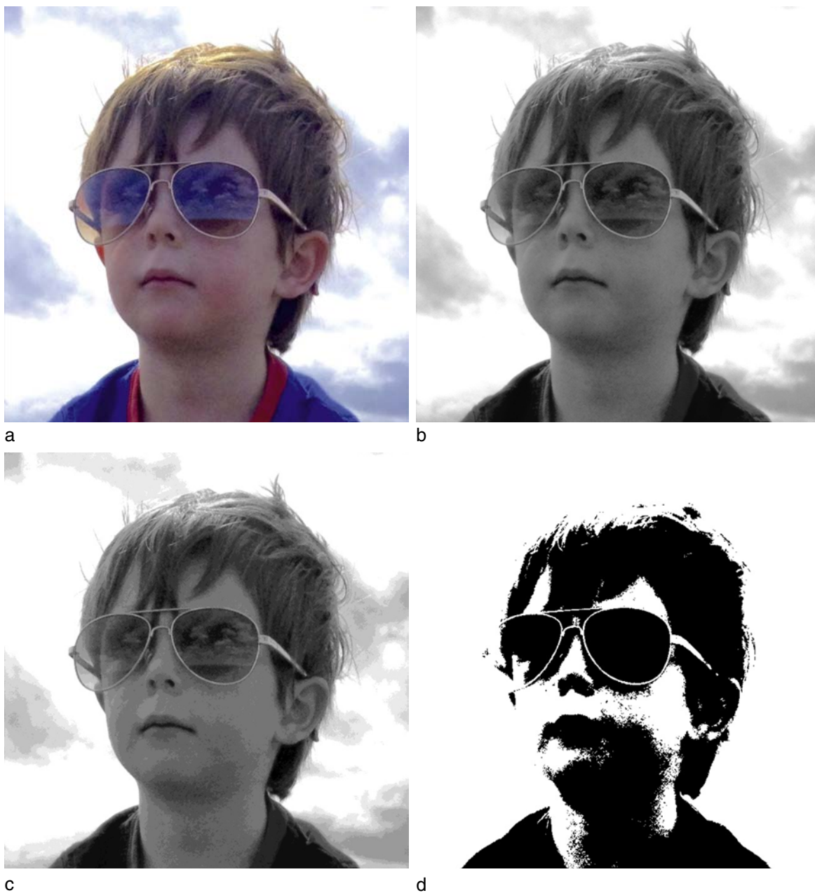
Fig. 22.1 When considering how images are represented 'perfect' fidelity may not be needed to convey meaningful information. The same original image is used throughout a-d . (a) A 'normal' full color image as produced by most conventional digital cameras. (b) The image modified to 256 shades of grey. (c) The image represented as only 16 possible shades of grey with a much reduced file size, but some discernible loss of image quality. (d) With only 2 possible values per pixel, the image is still recognizable and able to convey meaning, although it is significantly simplified and with a small fraction of the file size. (© Jonathan Bury)
