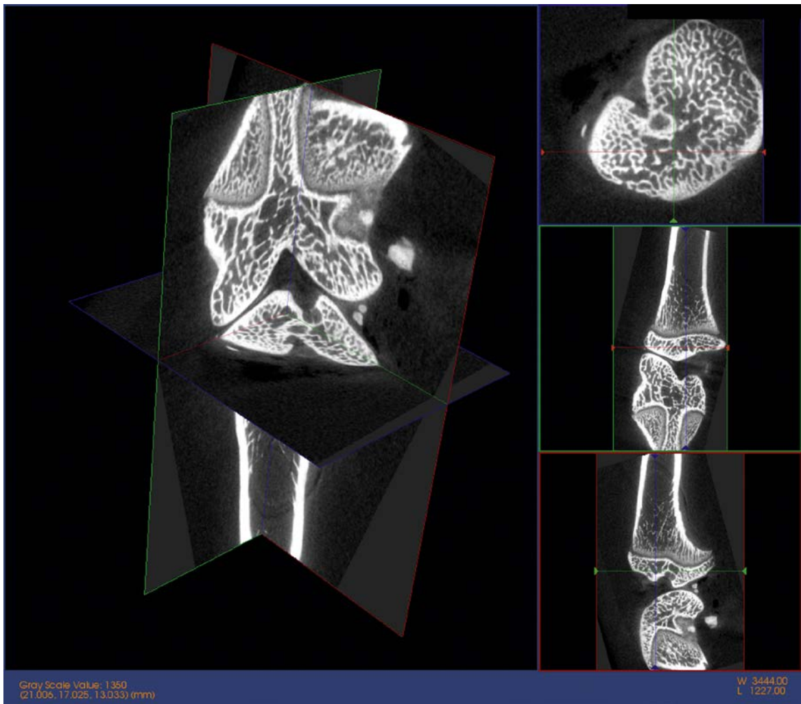
Fig. 17.14 Example of a specimen CT scan showing different dimensional measurement capabilities.
