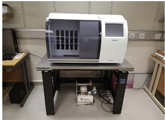
Fig. 22.3 This high-capacity high speed scanner (Philips UFS) has been installed on a vibration-damping table to minimize artifact from a railway line running very close to the laboratory. (Courtesy of Tristan Brain.)
