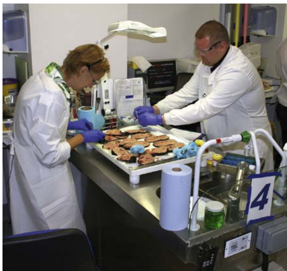
Fig. 5.1 A pathology dissection station with a downdraft ventilated bench and clear dissection zone. Note the well-lit and ergonomic layout for the grossing pathologist and the technician support. (Grateful thanks are expressed to Dr Caroline Verbeke and Mr Jonathan Sheriff for their assistance and consent for the illustration.)
