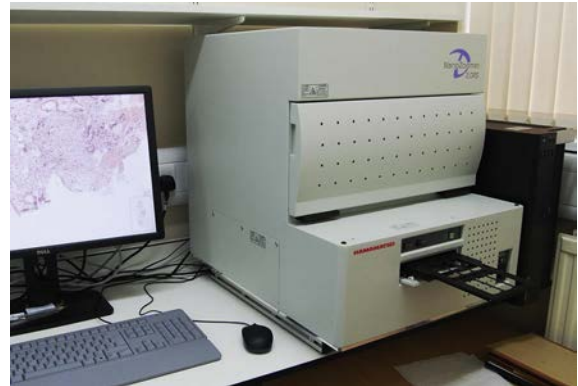
Fig. 22.6 This Hamamatsu scanner is used for capturing images for intraoperative frozen section diagnosis. The system holds just 6 slides but offers fast scan times which is appropriate for this application.
