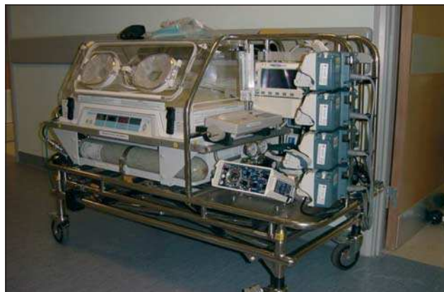
Neonatal transport system—mobile intensive care unit for safe and comfortable transport of infants
