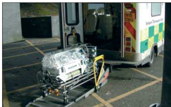
Loading mechanism for loading transport incubators into ambulances. All transport systems must meet regulation standards
