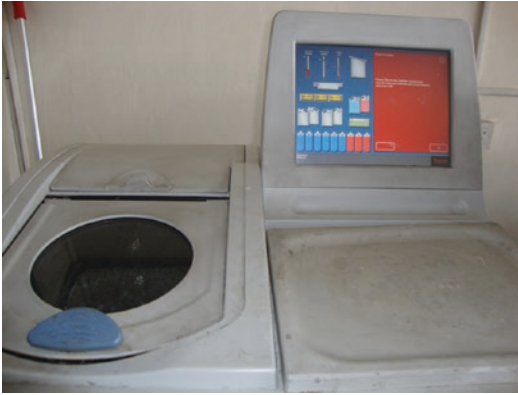
Fig. 2.3 Fluid transfer advanced automatic tissue processor. Here the fluid itself is changed automatically, and the bucket remains static
