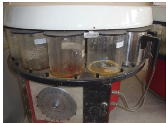
Fig. 2.2 Tissue transfer automatic tissue processor. Here the whole bucket containing tissue is automatically transferred to the next fluid station
