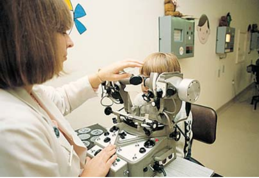
Figure 14.1. The synoptophore. An instrument for measuring the angle of deviation of a squint and the ability of the eyes to work together. □
